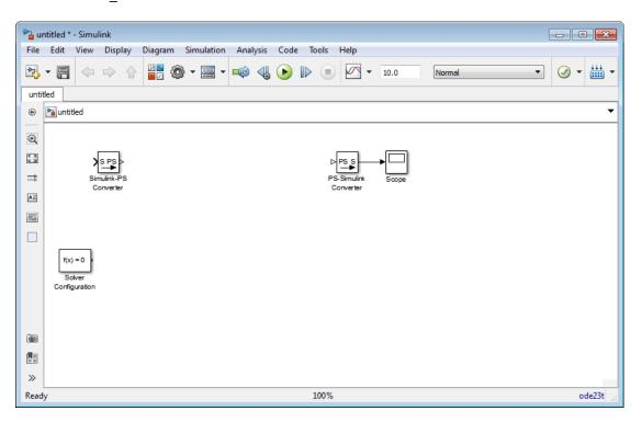
The new untitled model, with the default solver set to ode23t, contains a Solver Configuration block, a Simulink-PS Converter block, and a PS-Simulink Converter block connected to a Scope block.
