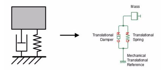
When constructing your network, it is important to include domain-specific reference blocks, such as Electrical Reference, Mechanical Translational Reference, and so on. Depending on domain, these blocks represent connection to ground, frame, or atmosphere. For more information, see "Grounding Rules".
